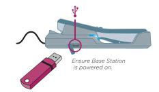
Insert USB drive into the USB port in the Base Station
